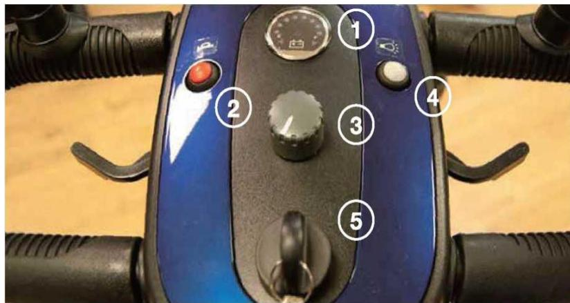
1. **Battery Gauge:** This gauge gives you a guide to the amount of charge left in the scooter's batteries. This will give the truest reading when the scooter is in motion.
